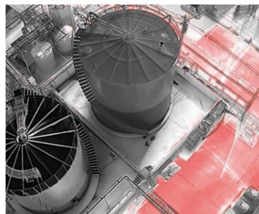
Infrared imaging of liquid levels inside the tank
